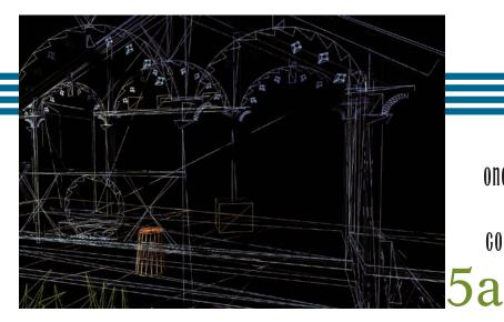
In the technique of vector lighting, one presets the lighting in the computer model and then through a set of commands assigns the lighting qualities to each vector.
